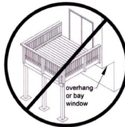
Figure 18. No Attachment to House Overhang with Ledger.
